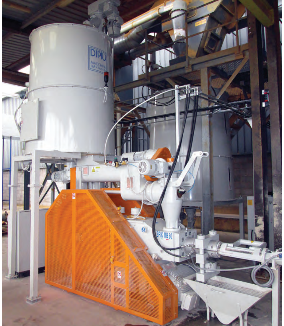
ENERGY BY VOLUME: Schumacher and his team ultimately decided the DiPiu MB80 was the right fit to bring compressed log manufacturing to Superior Pellet Fuels. Schumacher says the machine is currently yielding around 1 ton per hour of production.
